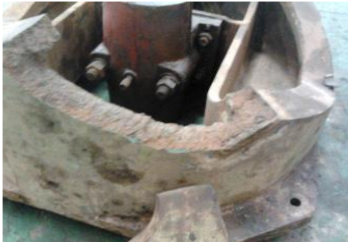
Figure 1 - Broken lifting pedestal
