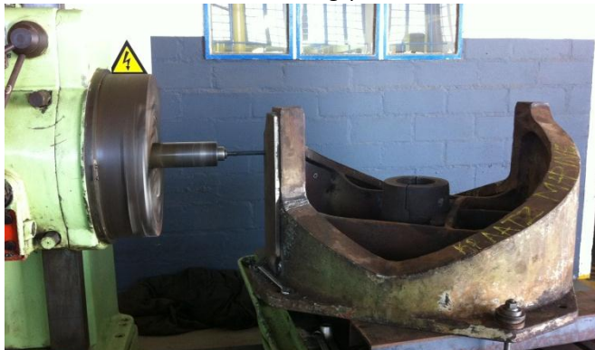
Figure 1 - Drilling of lifting pedestal
