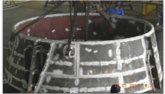
Figure 2 - After Non Destructive Testing (NDT)
