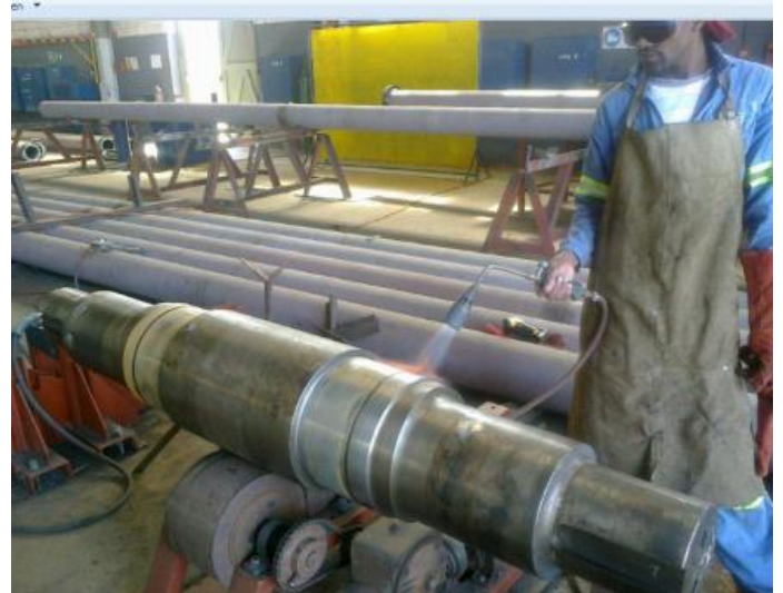
Figure 2 - Equal Soak preheating on Rotator
