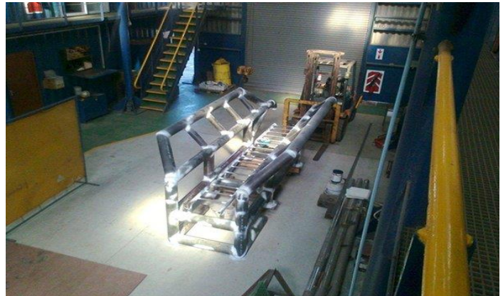
“Assembly, welding and NDE complete ready for painting”
